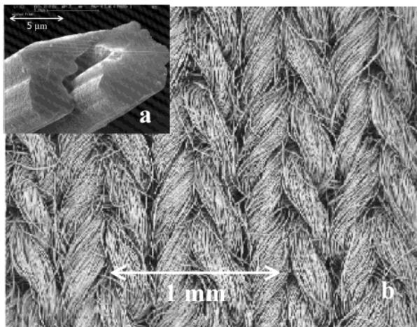
**Figure 1.** SEM image of a single fiber (a) and the knitted silica-fiber support (b).
